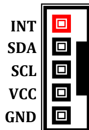
FIGURE 2-7: DMMEGA128A.Net 5 Pins Header I2C Interface.
