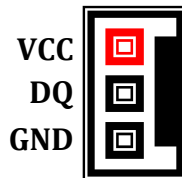
FIGURE 2-6: DMMEGA128A.Net Header 1 Pin 1 Wire Connector.
